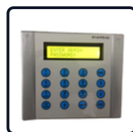
Access OTP Keypad
